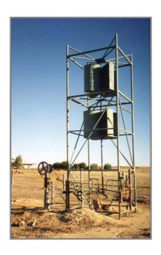
Savonius type WTGs have a vertical axis with usually four shovel-like blades. These are automatically always, in the wind', making complecated, yaw mechanisms' that keep horizontal WTGs in the direction of the wind unnecessary. Savonius type WTGs are easy to construct and need little maintenance. In Indonesia some exist for water pumping.
